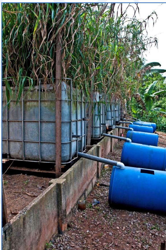
Figure 1: Pilot scale faecal sludge planted drying beds
