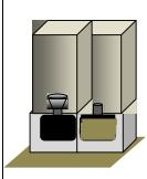
This UD option has two separate storage compartments for dry faeces that are used for alternate years. The compartments are emptied only after a year of storage by which time the faeces will have safely converted into an odourless dry humus, free of pathogens. It is then either buried or used as compost. This option is much more robust and 'user friendly' as compared to the above Bucket Type. Although initial capital outlay is higher there is theoretically no limit to the life of such systems.
