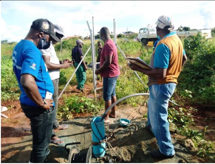
Borehole capacity test in progress at one of the newly drilled borehole sites - Emganwini, Emasotsheni
