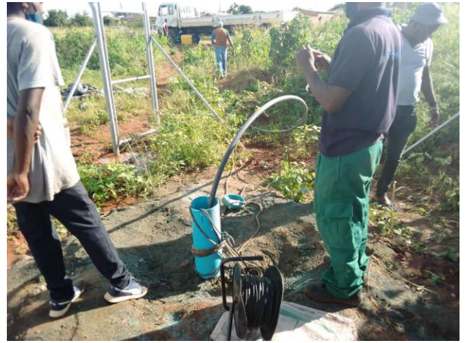
Borehole capacity test in progress at one of the newly drilled borehole sites - Emganwini, Emasotsheni
